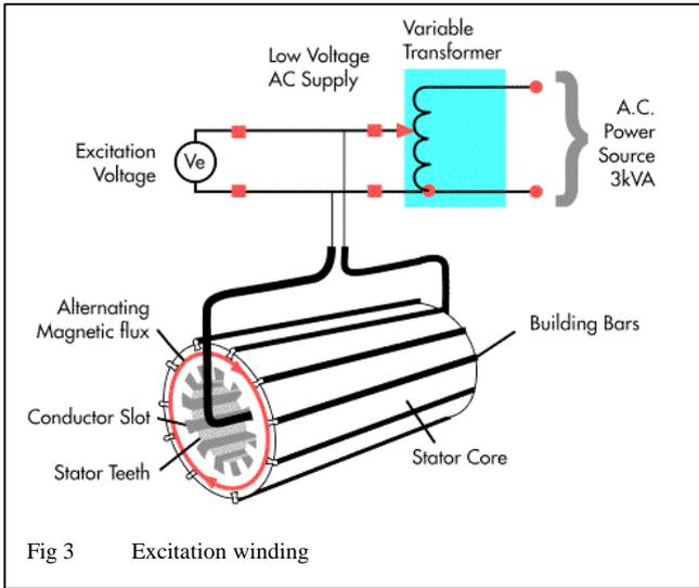
The eddy currents induced in any damaged areas are detected by sensing the magnetic fields resulting from them. Particularly for defects on or near the surface, their magnetic field extends beyond the surface and is detected by a sense coil applied across the teeth of the core.
