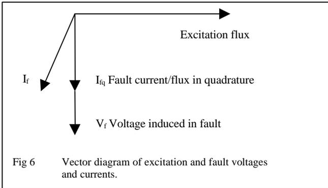
This reference should in principle be derived from a measurement of the core flux. However an adequate signal can be derived from the excitation current (which is in phase with the flux), sensed by a current probe whose output is in phase with the excitation current.
