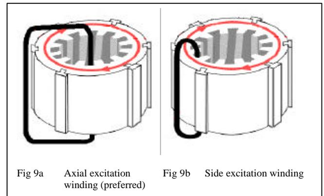
Fig 9a Axial excitation winding (preferred)
