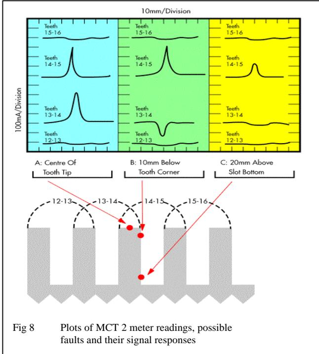
Fig 8 Plots of MCT 2 meter readings, possible faults and their signal responses
