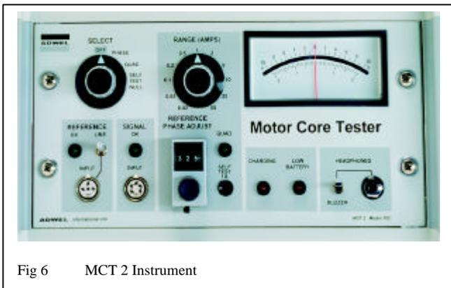
The centre-zero meter allows for positive and negative quad signals to be displayed, which is important in diagnosing the precise location of a fault. In addition the increase or decrease of signal is indicated in headphones by a variation in tone pitch. This use of “old fashioned” analogue indications and tone signals is due to the need to find maxima and minima, where digital indicators are less easy to read.
