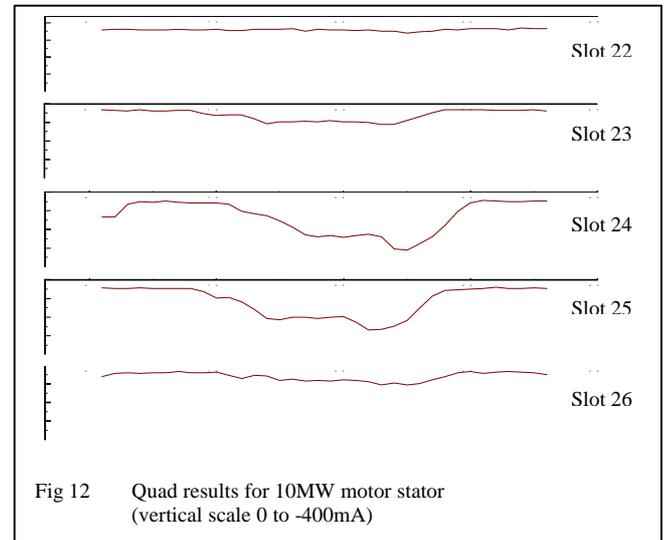
Fig 12 Quad results for 10MW motor stator (vertical scale 0 to -400mA)
