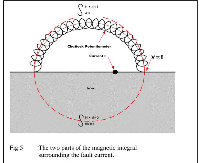
Fig 5 The two parts of the magnetic integral surrounding the fault current.
