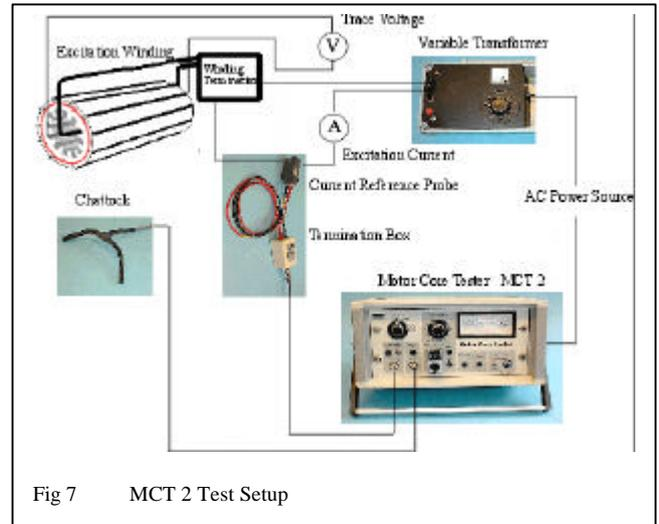
A section of the core that is assuredly not defective (determined by cross-checking at several different points) is tested by bridging a pair of teeth with the chattock, and adjusting the MCT 2 reference phase adjust to trim the quad signal to zero. This sets the phase sensitive discriminator ready for use.
