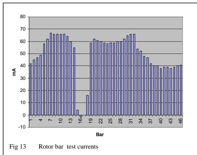
Fig 13 Rotor bar test currents
