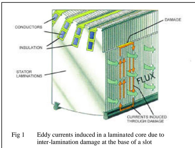
Fig 1 Eddy currents induced in a laminated core due to inter-lamination damage at the base of a slot
