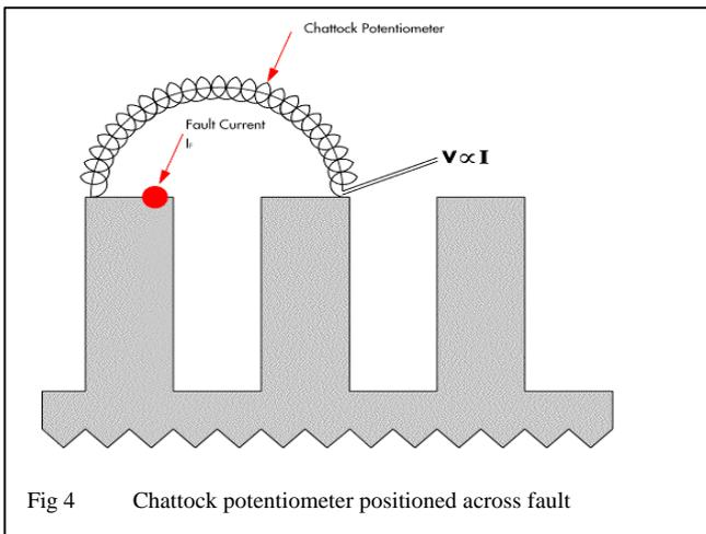
The ability of the Chattock to measure the actual fault current is due to Ampère's law that the integral of the magnetic field surrounding a current is equal to the current enclosed, shown in fig 5. In the situation of a chattock coil
